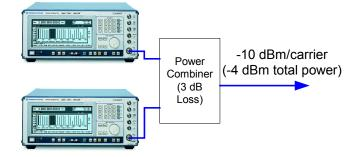
Fig. 6: Recommended simplified configuration using 2 SMIQs
