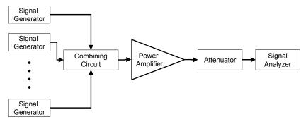
Fig. 1: Basic setup for ACLR measurements on a base station power amplifier stage.
