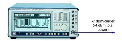
Fig. 2: Generating a 4-carrier 3GPP signal with a single SMIQ03HD
